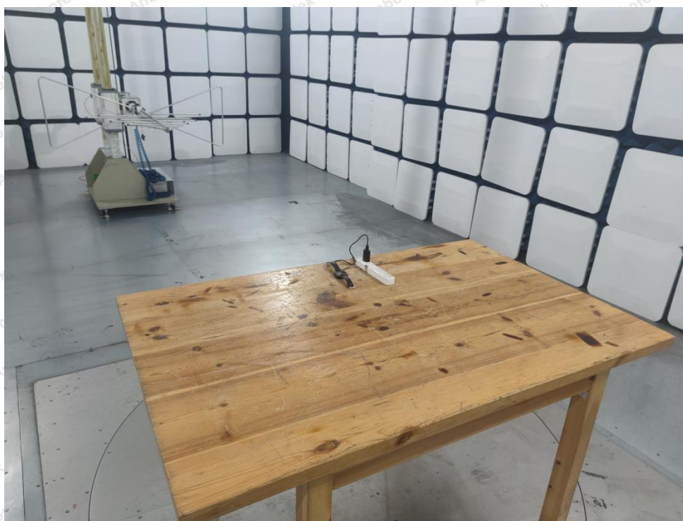
Photo of Radiation Emission Test
