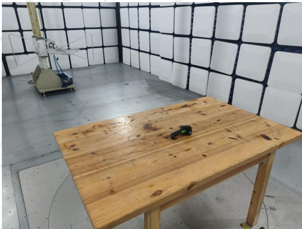
Photo of Radiation Emission Test
