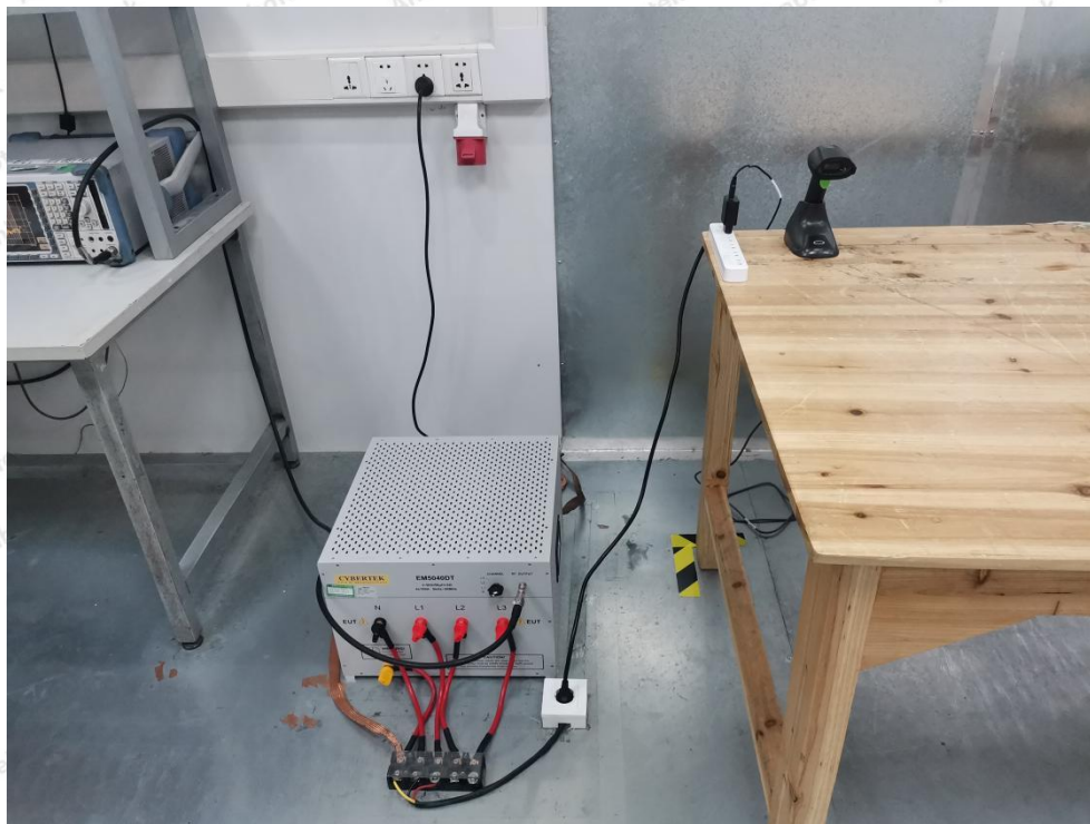
Photo of Conducted Emission Measurement
