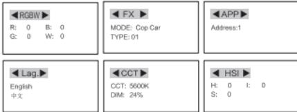
(1) In the RGBW mode interface, press the FN switch to switch between "R, G, B, W" setting.
