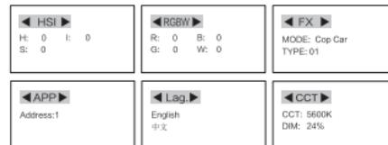
(1)In the HSI mode, turn the FN switch to cycle between " H, S, I " setting.
