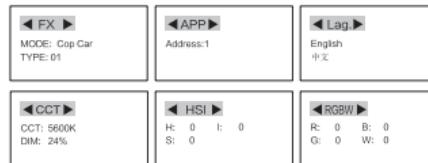
(1) In the FX (special effect) mode interface, turn the FN switch to switch between different scene modes setting as below:
