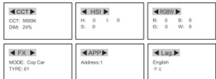
(1)In the CCT mode interface, turn the FN switch to adjust the color temperature between 3200K and 5600K.
