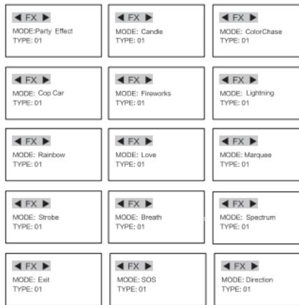
(2) In the FX (special effect) mode interface, press the FN switch to choose between type 1, 2 and 3 in the same scene effect. For example, type 1, 2, 3 in "party effect" means three different party effect. User can choose whichever according to the different shooting requirement.
