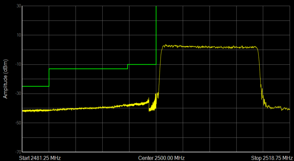
Band7 QPSK BW=15MHz Channel=20825 RB Size=75 Position=#0
