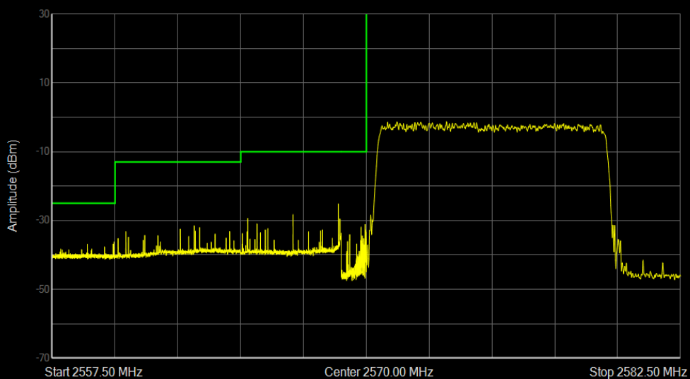
Band38 QPSK BW=10MHz Channel=37800 RB Size=50 Position=#0
