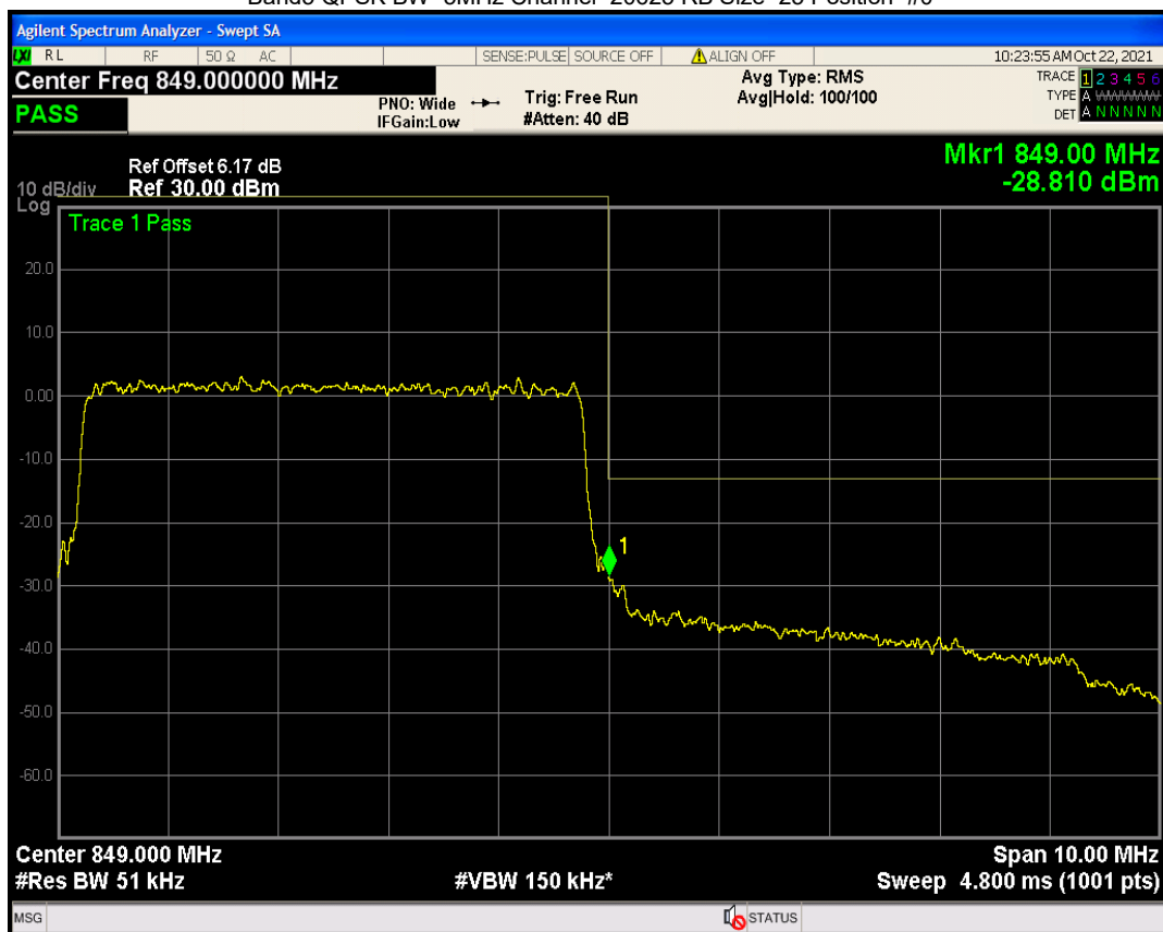
Band5 QAM16 BW=5MHz Channel=20625 RB Size=25 Position=#0
