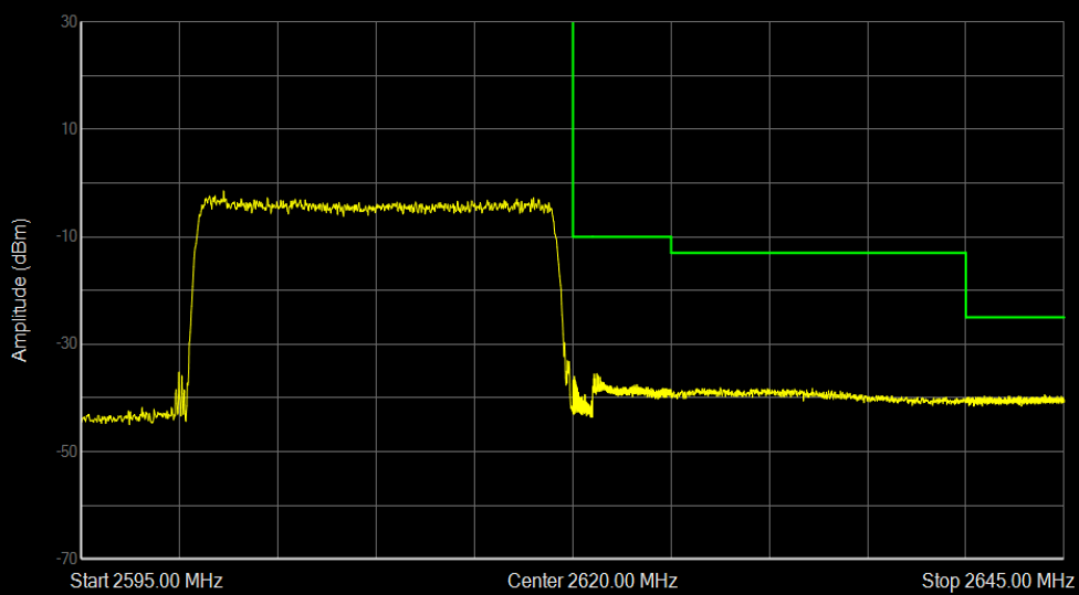
Band38 QPSK BW=20MHz Channel=38150 RB Size=100 Position=#0
