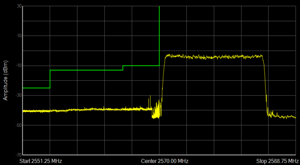
Band38 QPSK BW=15MHz Channel=37825 RB Size=75 Position=#0
