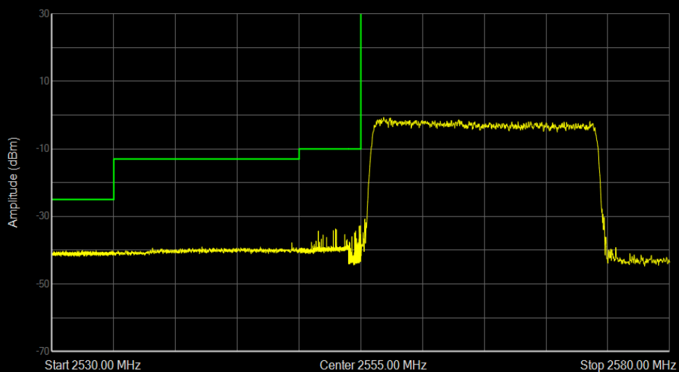
Band41(2555-2655) QPSK BW=20MHz Channel=40340 RB Size=100 Position=#0
