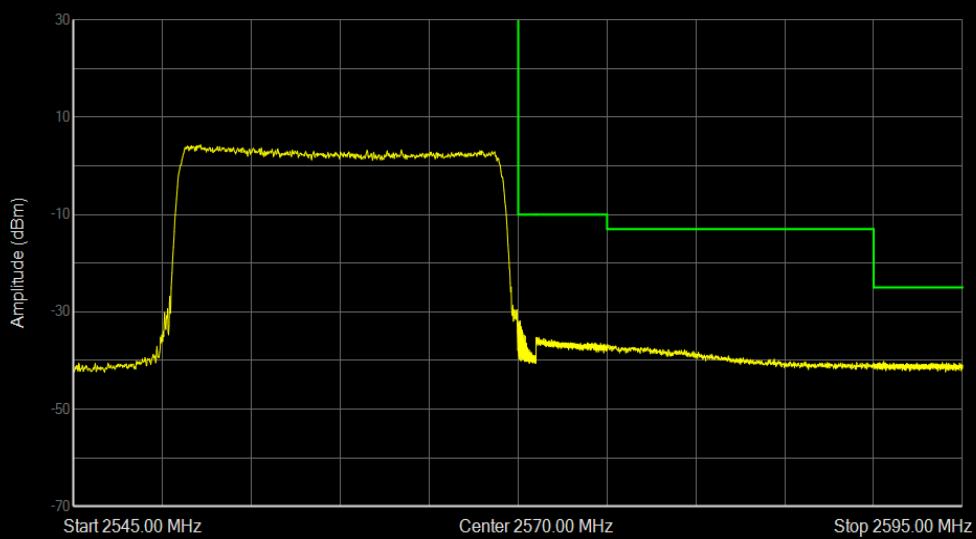
Band7 QPSK BW=20MHz Channel=21350 RB Size=100 Position=#0
