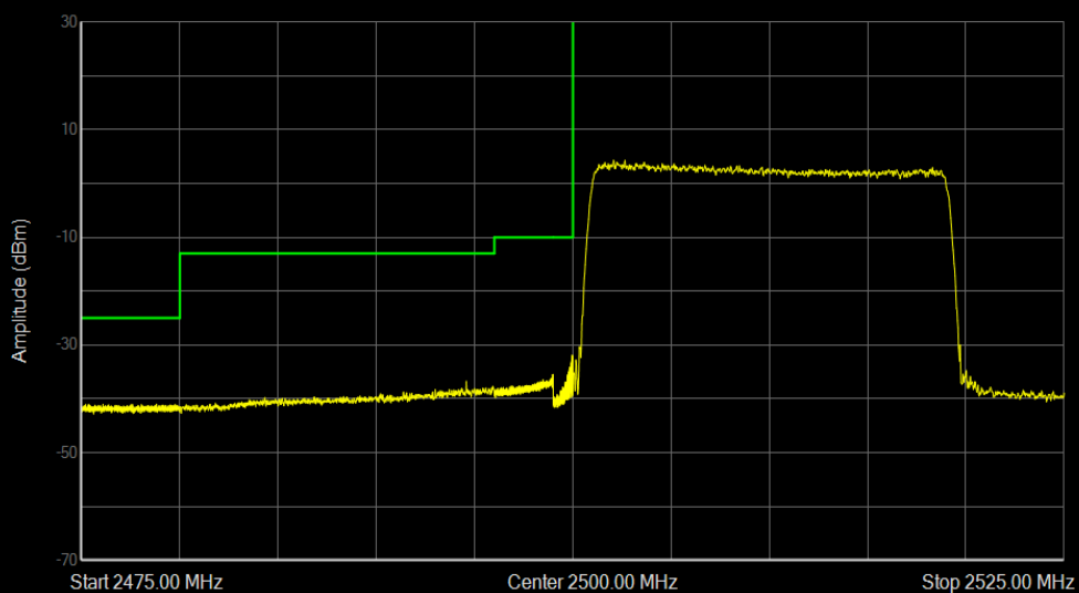
Band7 QPSK BW=20MHz Channel=20850 RB Size=100 Position=#0
