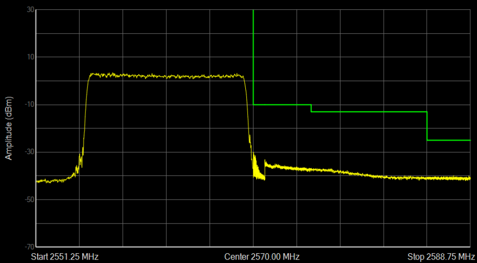
Band7 QPSK BW=15MHz Channel=21375 RB Size=75 Position=#0
