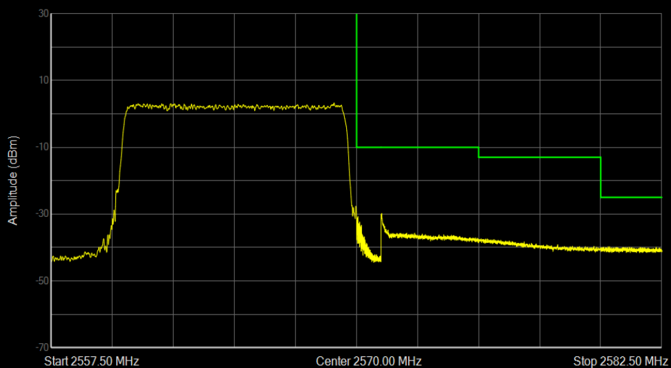
Band7 QPSK BW=10MHz Channel=21400 RB Size=50 Position=#0
