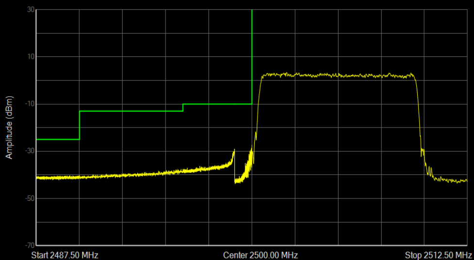
Band7 QPSK BW=10MHz Channel=20800 RB Size=50 Position=#0
