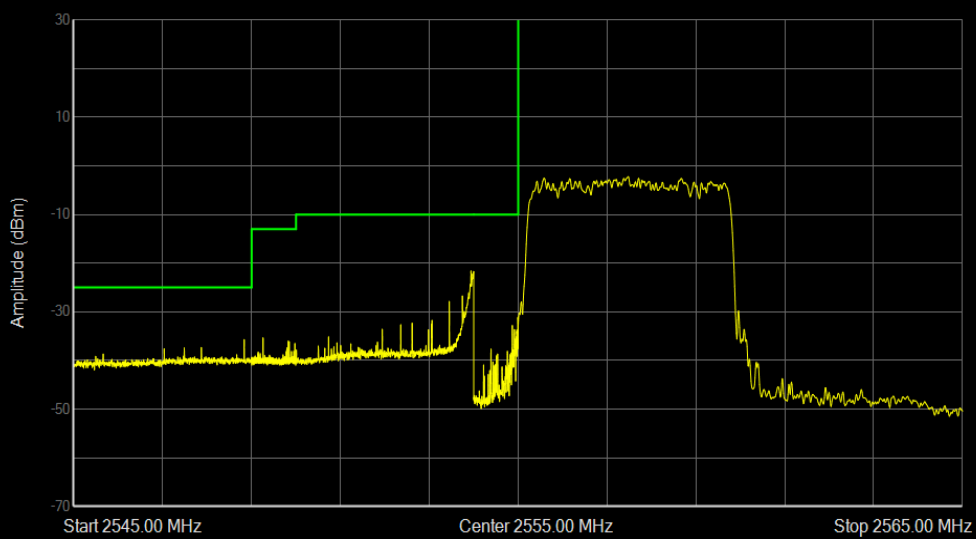
Band41(2555-2655) QPSK BW=5MHz Channel=40265 RB Size=25 Position=#0
