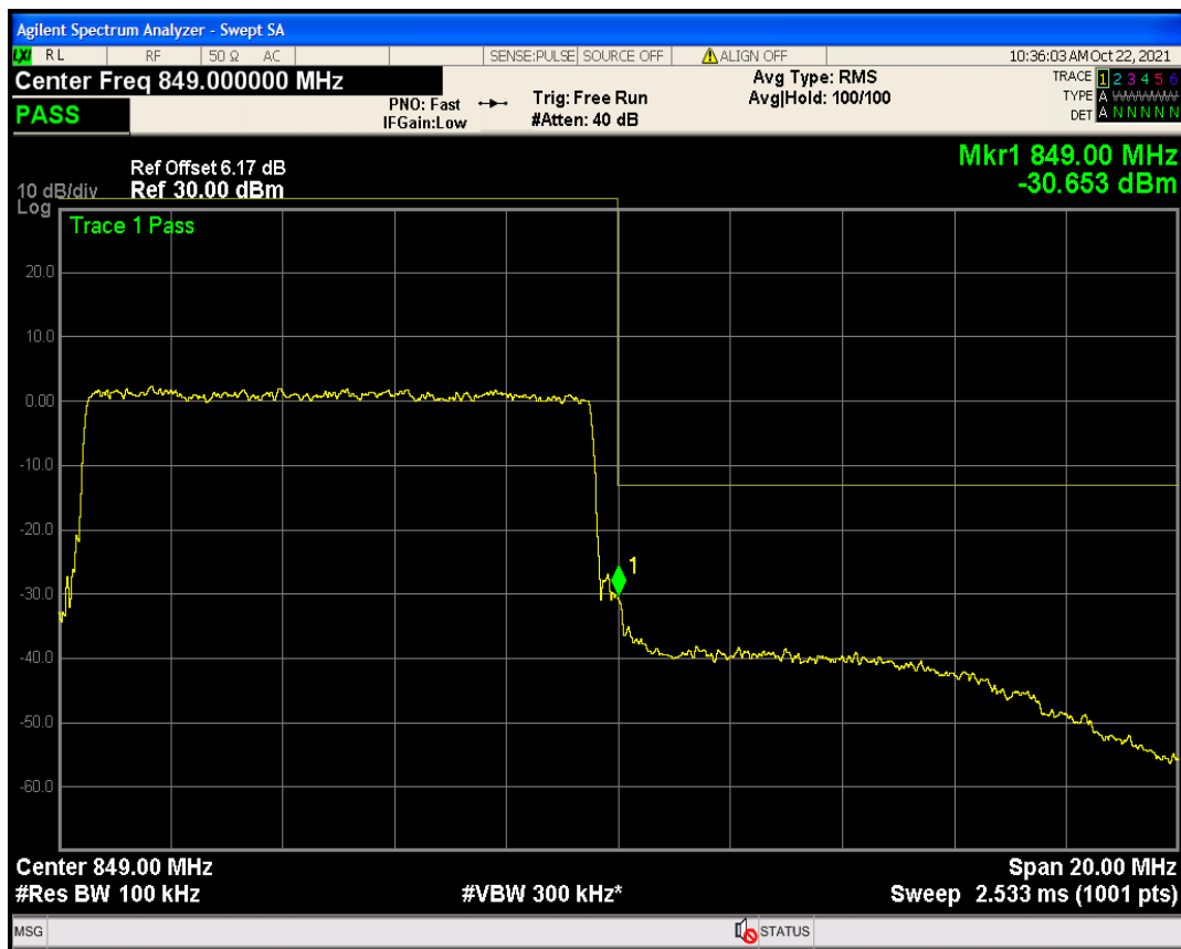
Band7 QPSK BW=5MHz Channel=20775 RB Size=25 Position=#0
