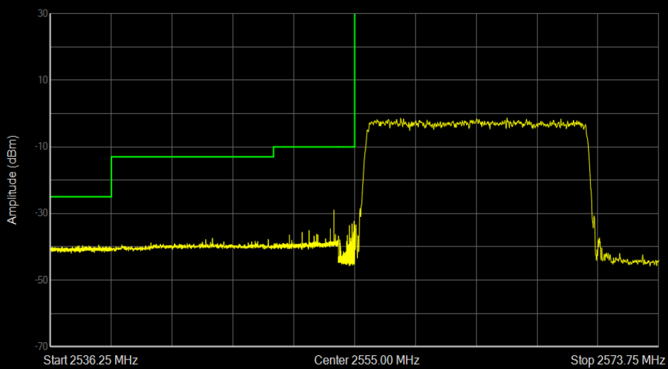
Band41(2555-2655) QPSK BW=15MHz Channel=40315 RB Size=75 Position=#0
