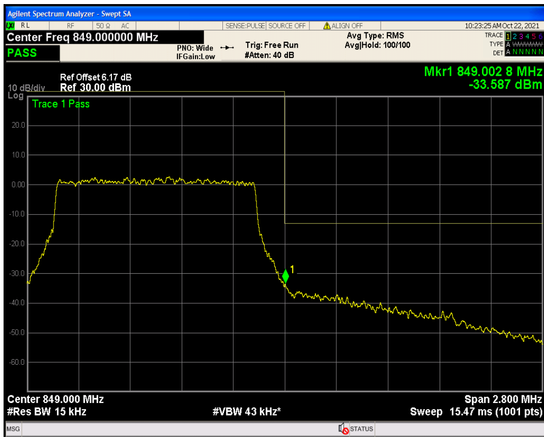
Band5 QPSK BW=3MHz Channel=20415 RB Size=15 Position=#0
