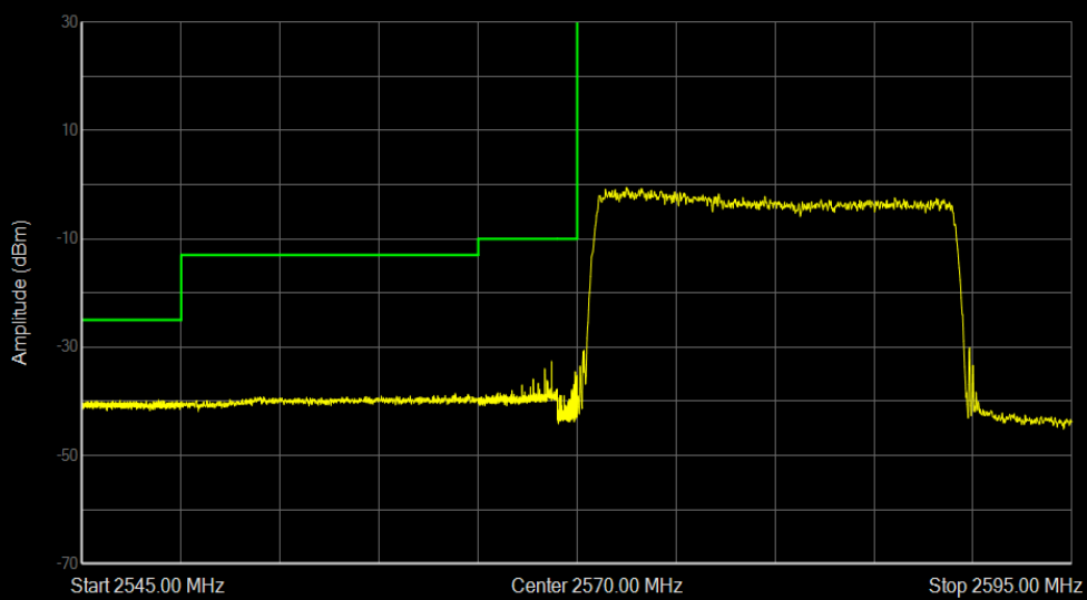
Band38 QPSK BW=20MHz Channel=37850 RB Size=100 Position=#0
