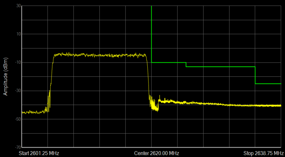
Band38 QPSK BW=15MHz Channel=38175 RB Size=75 Position=#0
