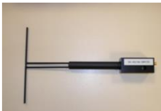
Figure 1 – MVG COMOSAR Validation Dipole
