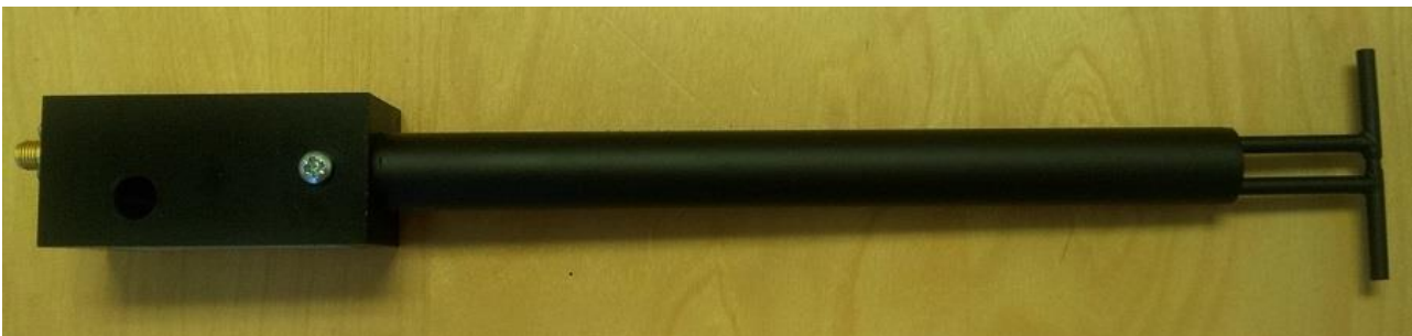
Figure 1 – MVG COMOSAR Validation Dipole
