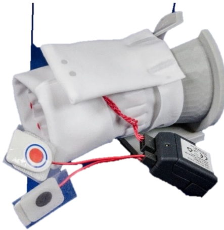
Setup for conducted disturbance emission test
