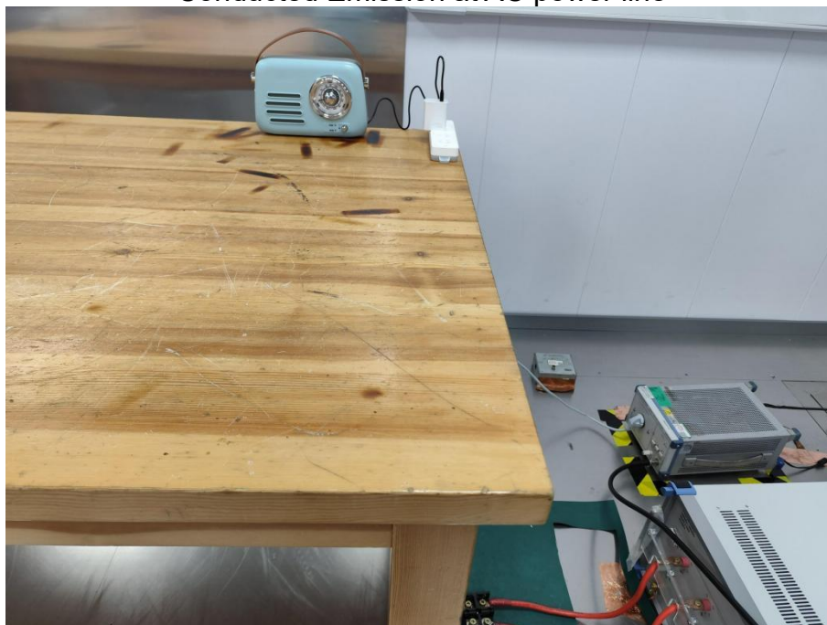
Conducted Emission at AC power line
