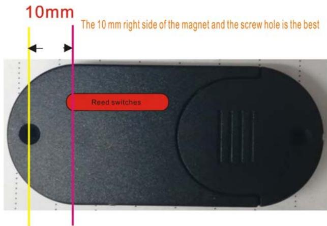
**Note: The magnet cannot be swept across from the beginning to the end between the two screws of the Bluetooth box, which may cause inaccurate transmission data.**
