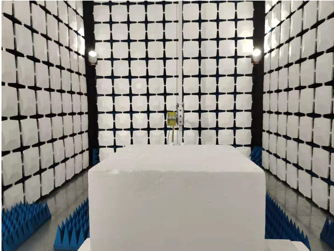
Above 1GHz for radiated emission test setup
