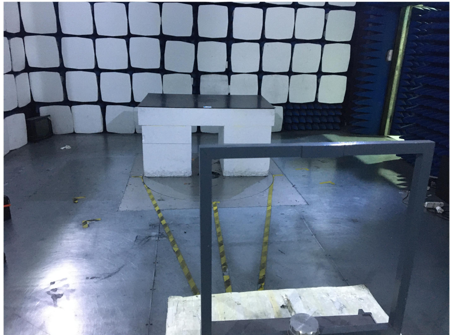
Radiation Emission Test Setup (Below 30MHz)
