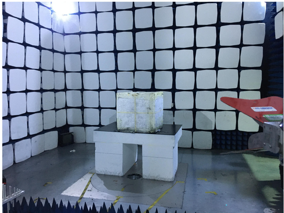
Radiation Emission Test Setup (1GHz to 18GHz)
