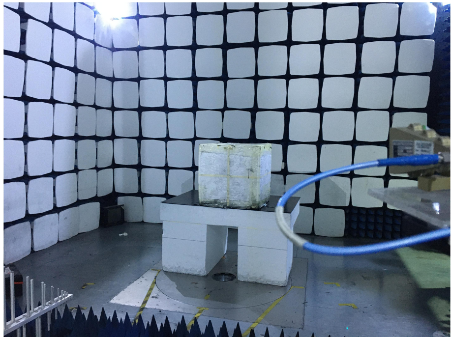
Radiation Emission Test Setup (Above 18GHz)
