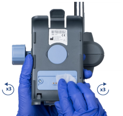
Figure 11.1. Cleaning Electric Connectors
