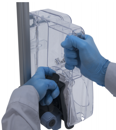
Figure 2.14. Removing the Lockbox from IV pole while using with Sapphire Connect
