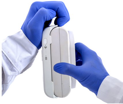
Figure 2.21. Releasing Sapphire Connect from Sapphire Pump
