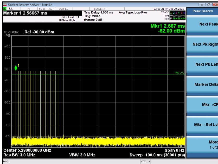
**Channel Move Time & Channel Close Transmission Time**
