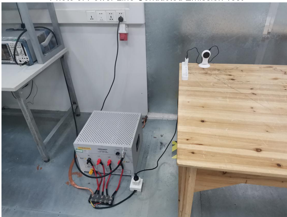
Photo of Power Line Conducted Emission Test
