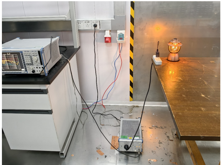
Conducted Emission Test Setup-TM1
