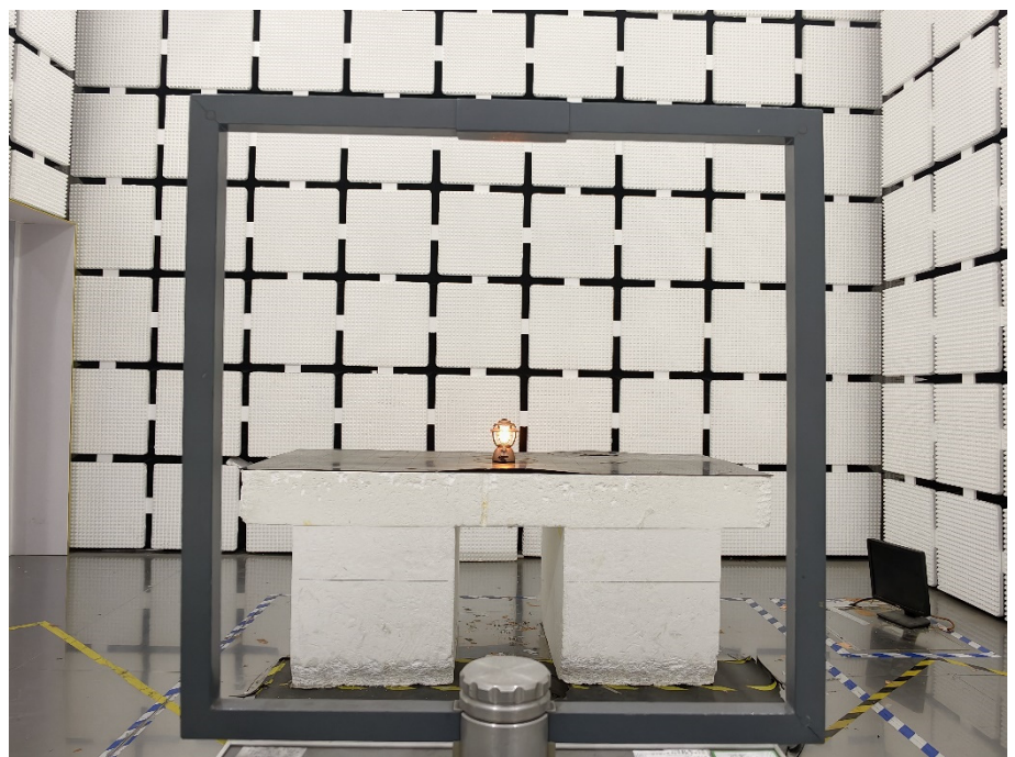
Radiation Emission Test Setup (Below 30MHz)
