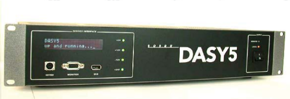
Photo of Server for DASY5
