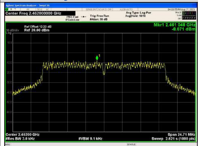
IEEE 802.11g_Channel 11_20MHz_Antenna 0
