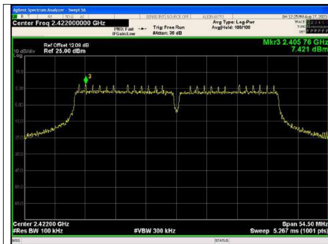
In-Band Reference Level IEEE 802.11n_Channel 3_40MHz_Antenna 0
