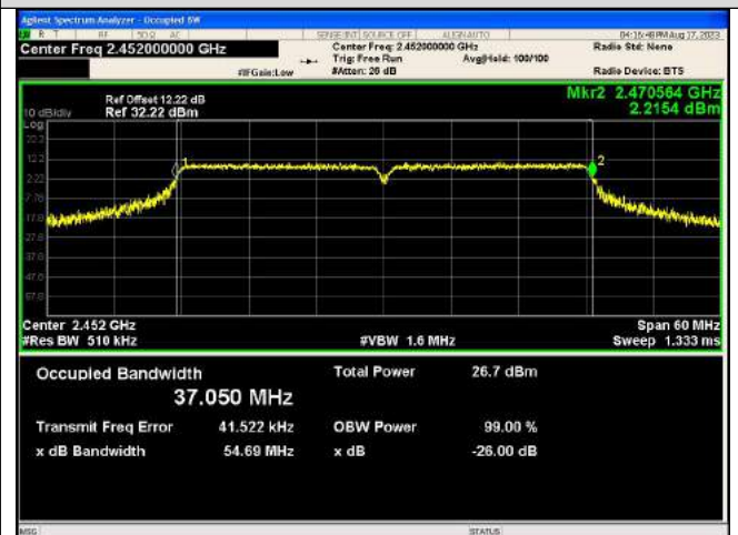
IEEE 802.11n_Channel 9_40MHz_Antenna 0
