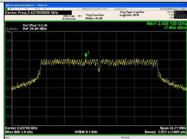
IEEE 802.11g_Channel 6_20MHz_Antenna 0
