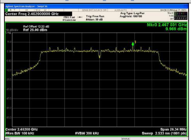
In-Band Reference Level IEEE 802.11n_Channel 11_20MHz_Antenna 0
