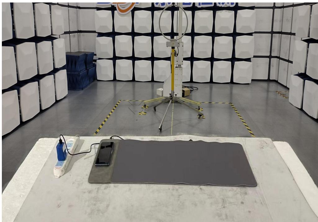
Conduction emission testing device
