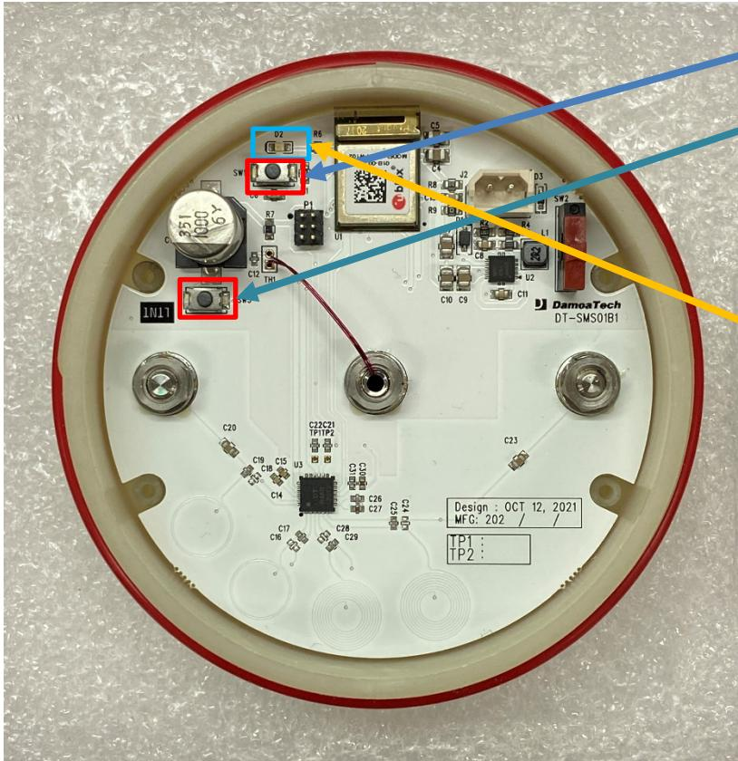
1. Switch at 11 o'clock = Power Reset button
