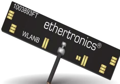
**BT Tunable FPC 2.4 GHz Embedded Antenna with cable**
