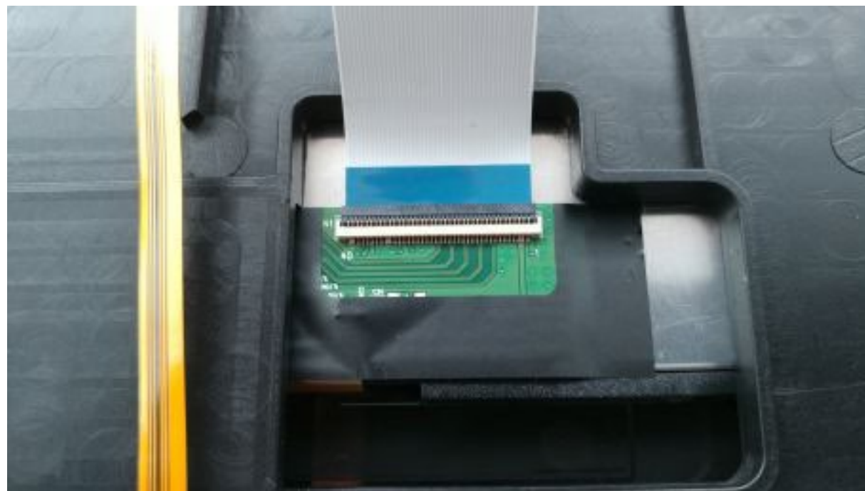
Figure 3-8: LVDS to LCD
