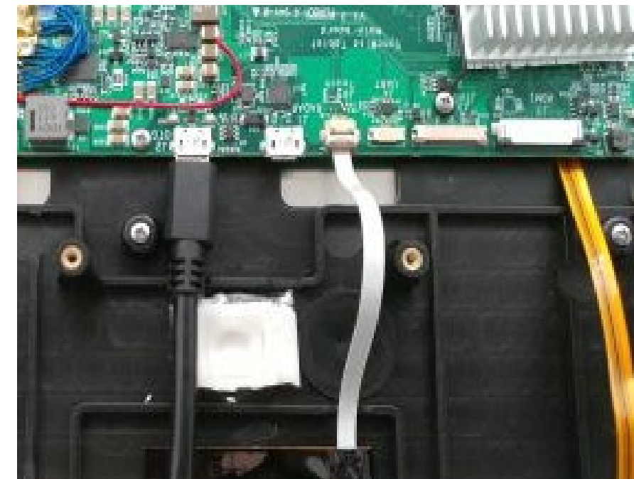
Figure 3-9: Touch cap FPC to PCB
