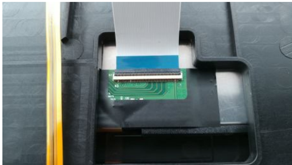
Figure 3-8: LVDS to LCD
