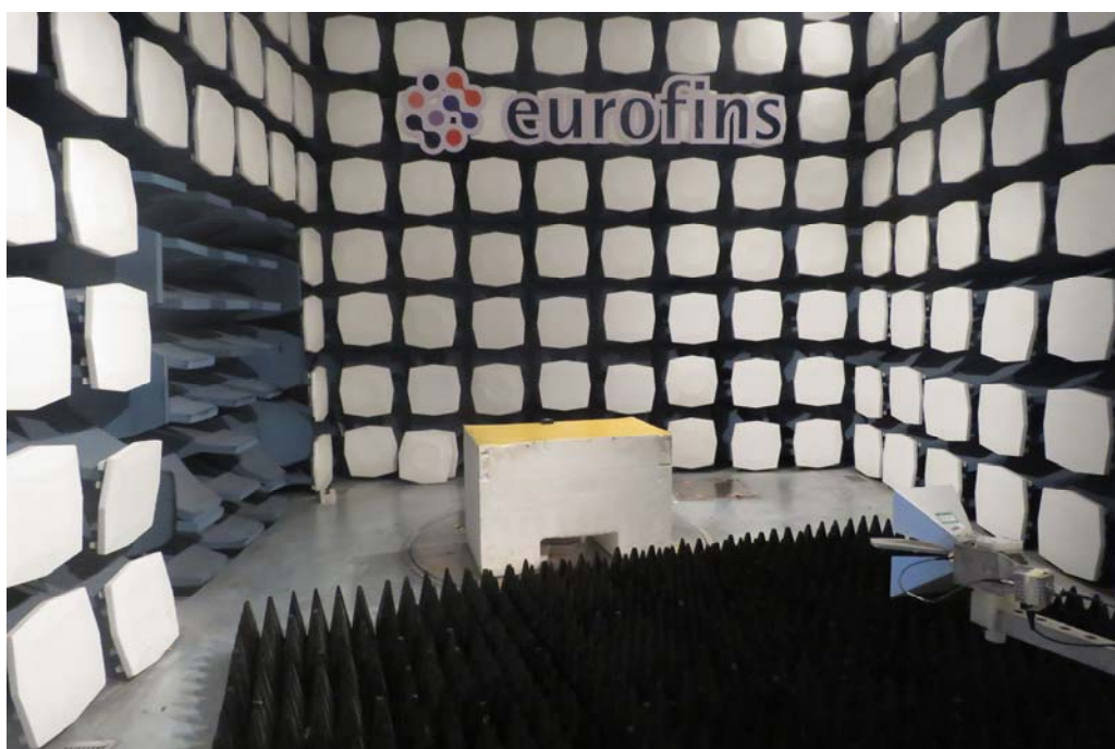
Picture 1: Radiated Emission Test Setup
