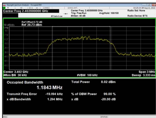
BT 2DH5 CH39, Carrier frequency (MHz): 2441
