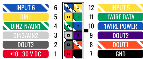
FMM230 2x6 socket pinout
