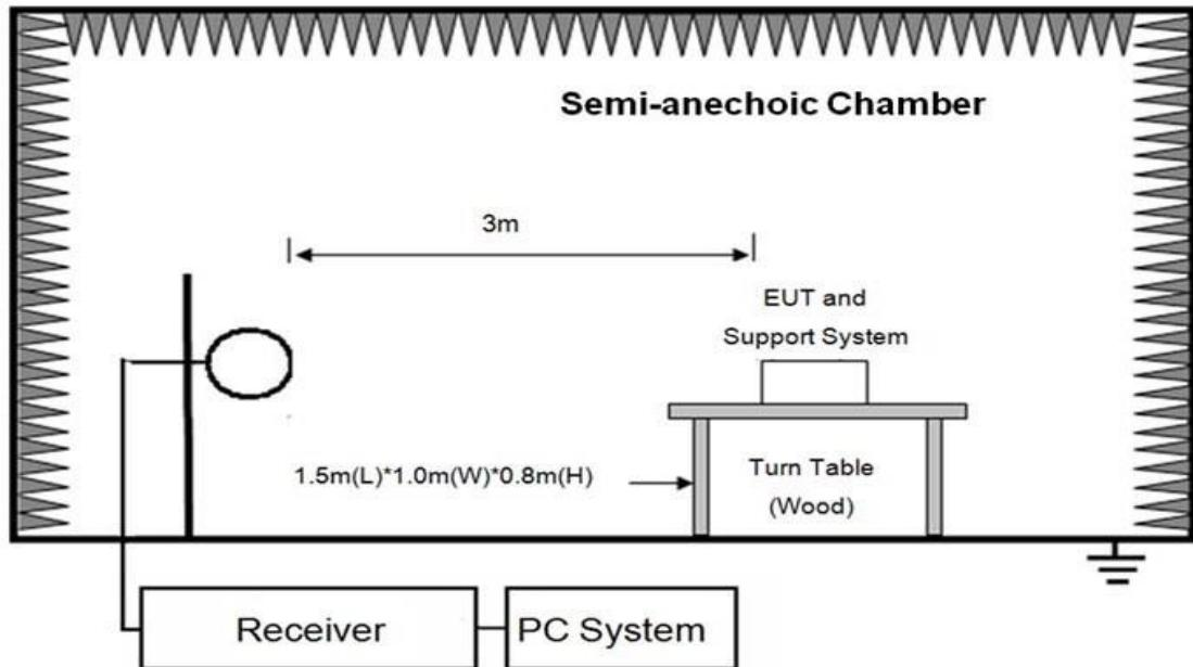
In 3m Anechoic Chamber Test Setup Diagram for 30MHz~1GHz
