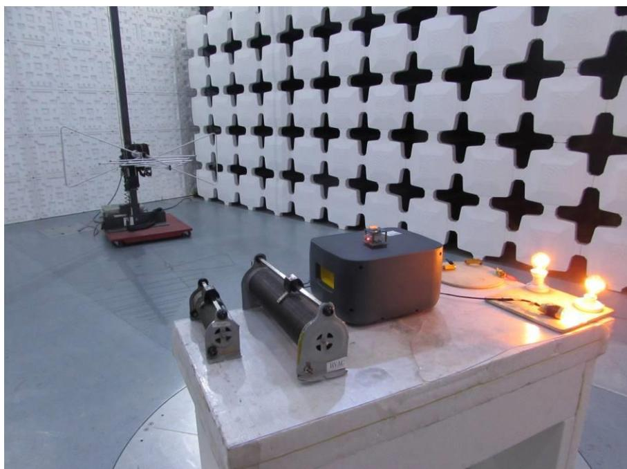
Conducted disturbance voltage at mains ports (150KHz-30MHz)
