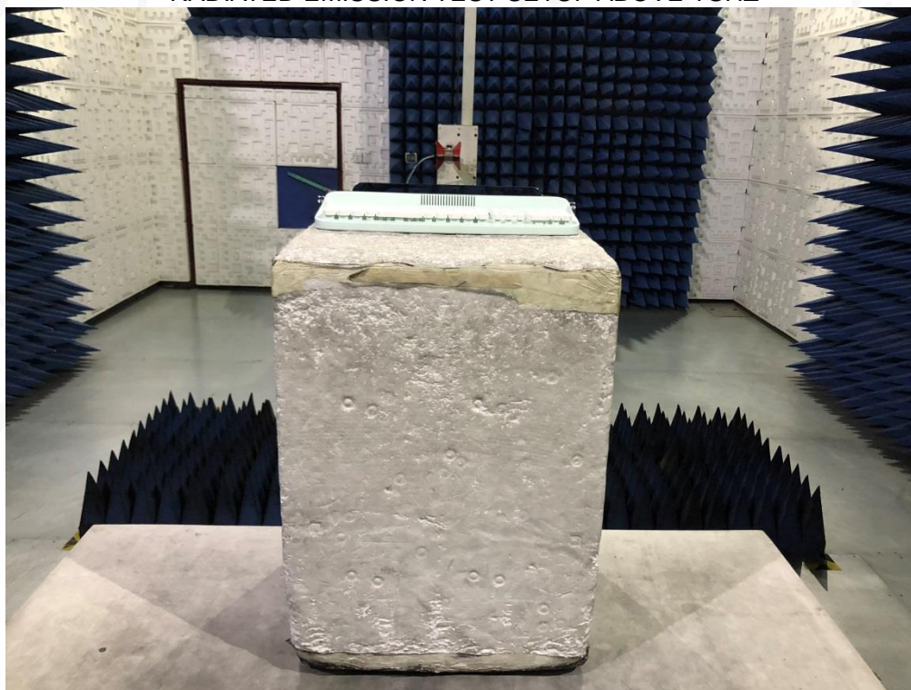
RADIATED EMISSION TEST SETUP ABOVE 1GHZ
