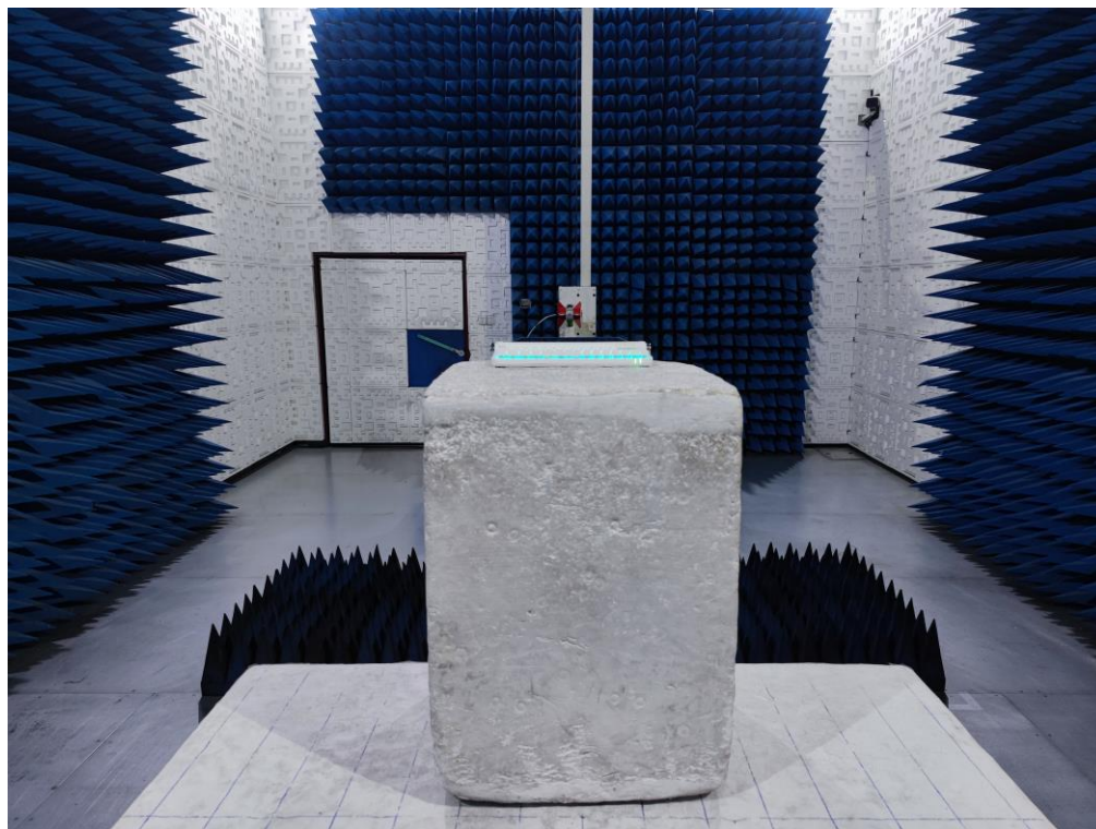
RADIATED EMISSION TEST SETUP ABOVE 1GHz
