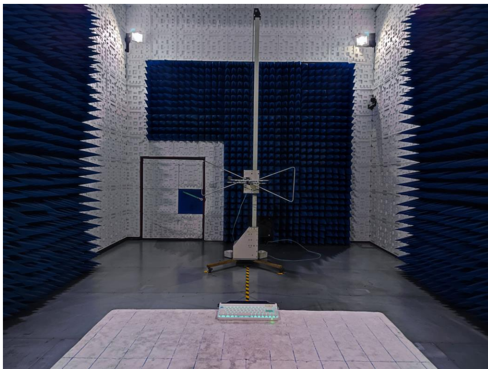
RADIATED EMISSION TEST SETUP ABOVE 1GHz
