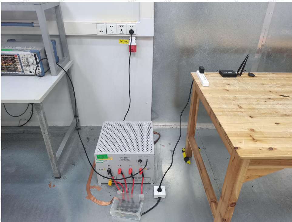
Photo of Conducted Emission Measurement
