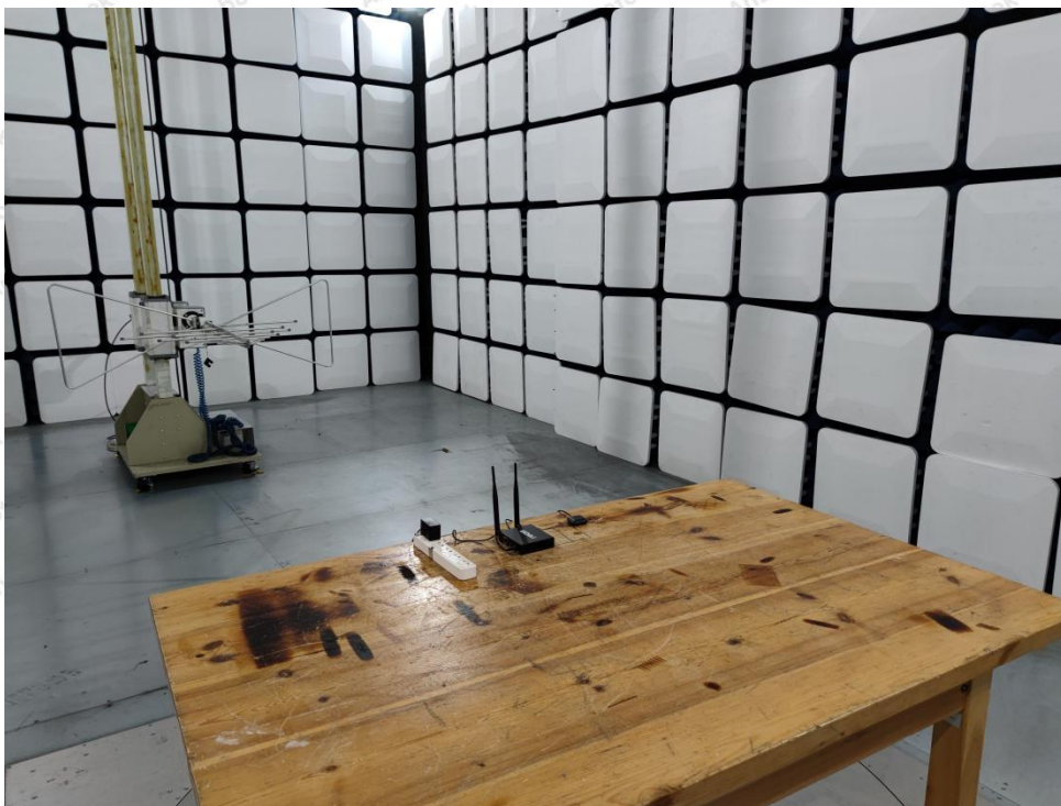
Photo of Radiation Emission Test
