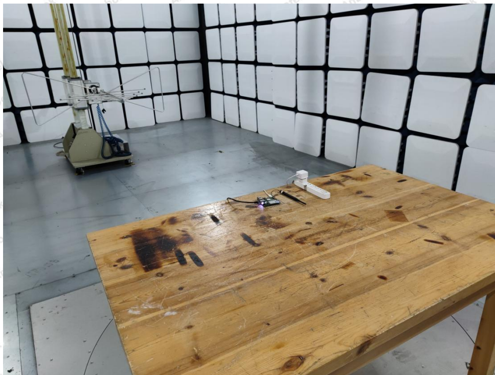
Photo of Radiation Emission Test
