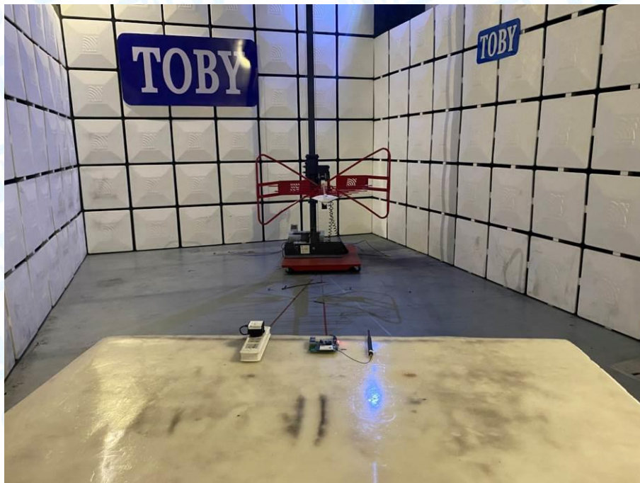
Photo of Setup for Conducted Emission
