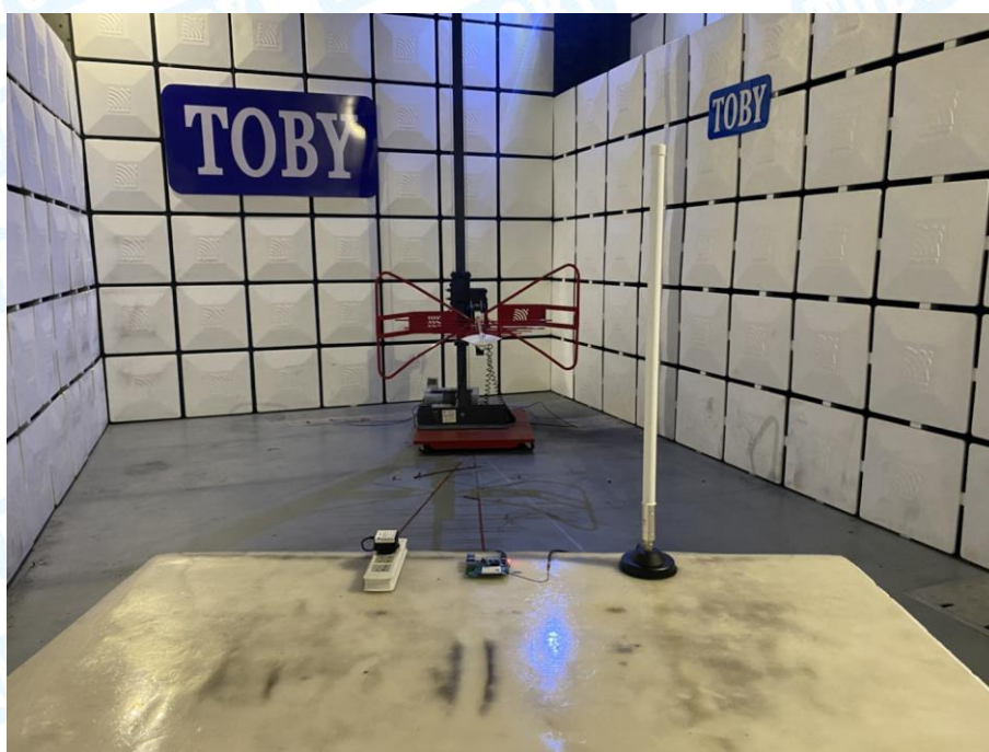
Photo of Setup for Radiated Emission (Below 1 GHz) ANT.2
