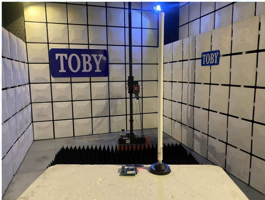
Photo of Setup for Radiated Emission (Above 1 GHz) ANT.2
