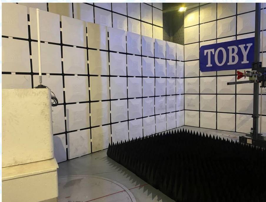
Photo of Setup for Radiated Emission (Above 1 GHz) ANT.2
