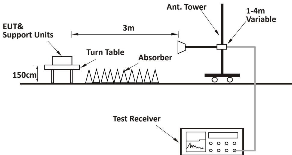
**TEST REPORT****7.4 Test Results of Radiated Emissions**
