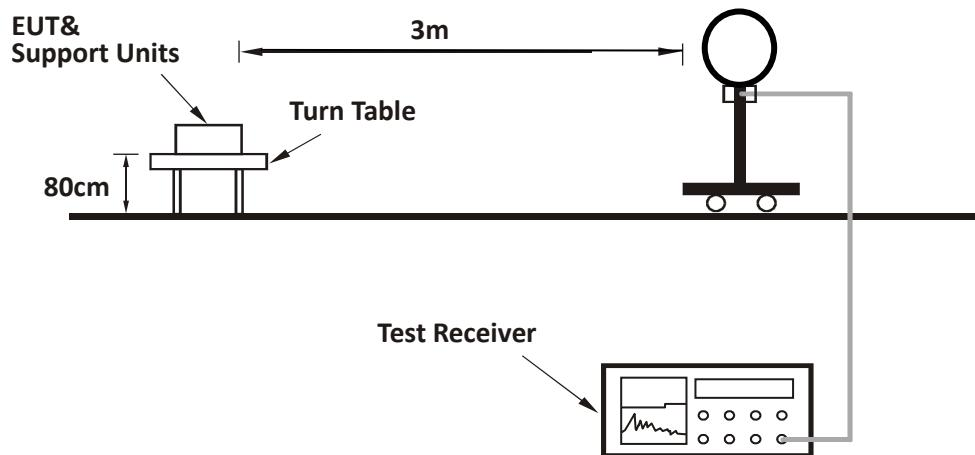
**For Radiated emission 30MHz to 1GHz:**
