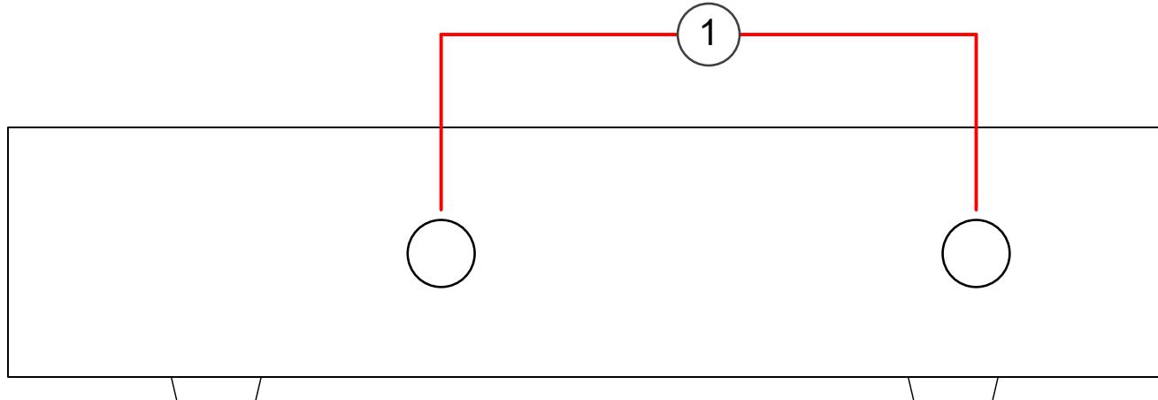
**1** LTE antenna connector (two on each side)
