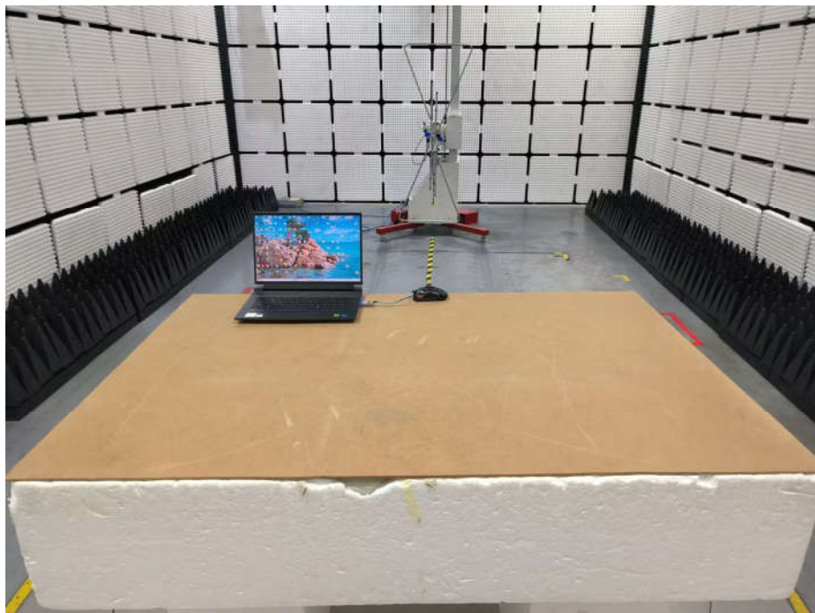
Radiated spurious emission Test Setup-1(Below 1GHz)
