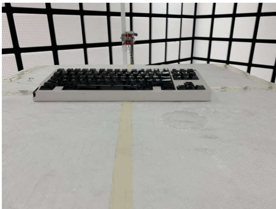
Radiated spurious emission Test Setup-2(Above 1GHz)
