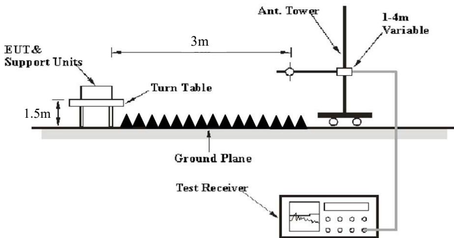
The radiated emission performed in the 3 meters, using the setup accordance with the ANSI C63.10-2013. The specification used was the FCC 15.209, FCC 15.247 limits.
