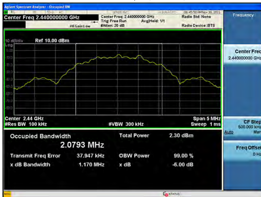
6 dB Bandwidth plot (Mid-CH 19)
