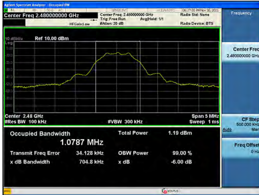
6 dB Bandwidth plot (High-CH 39)
