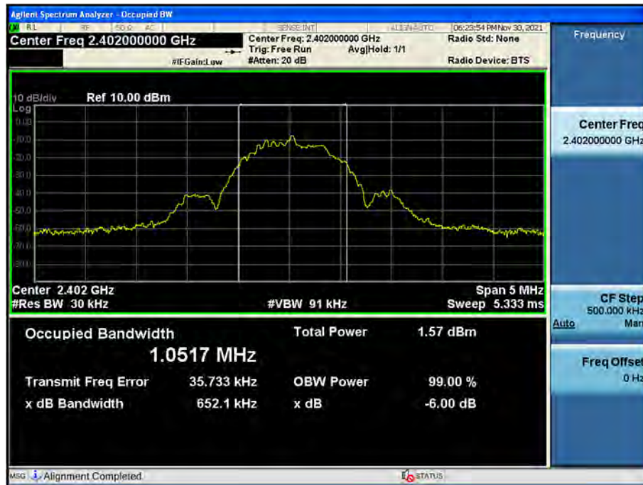
99 % Bandwidth plot (Low-CH 0)
