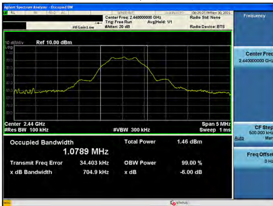
6 dB Bandwidth plot (Mid-CH 19)
