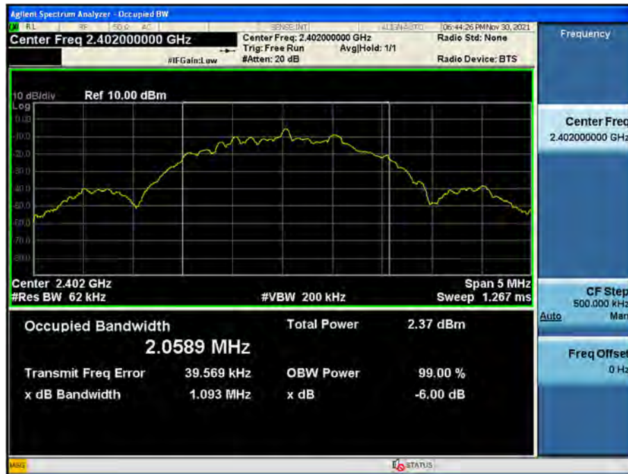
99 % Bandwidth plot (Low-CH 0)
