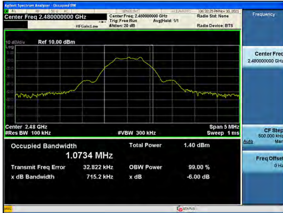
6 dB Bandwidth plot (High-CH 39)
