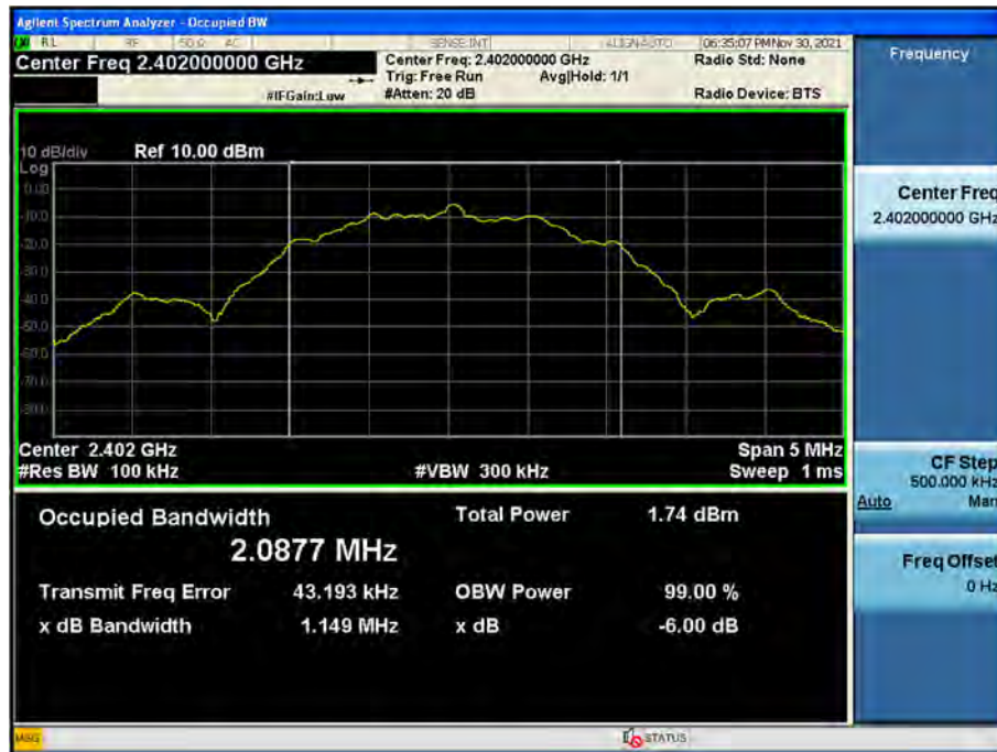
6 dB Bandwidth plot (Low-CH 0)
