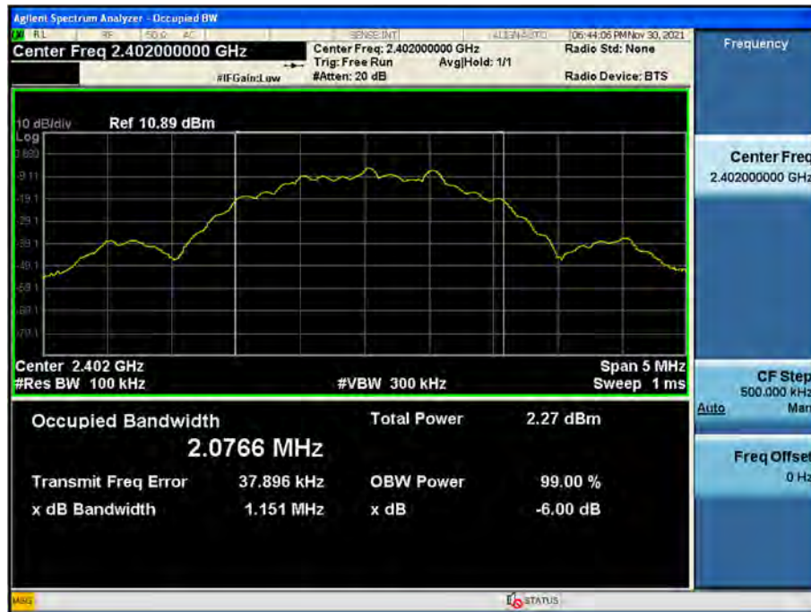
6 dB Bandwidth plot (Low-CH 0)
