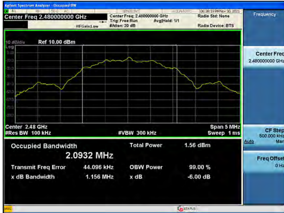
6 dB Bandwidth plot (High-CH 39)
