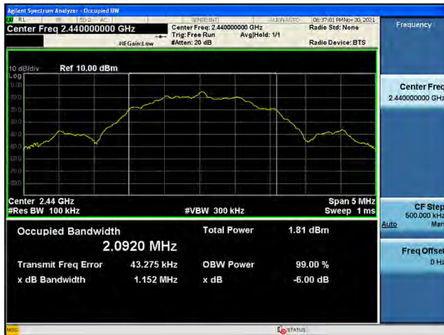
6 dB Bandwidth plot (Mid-CH 19)
