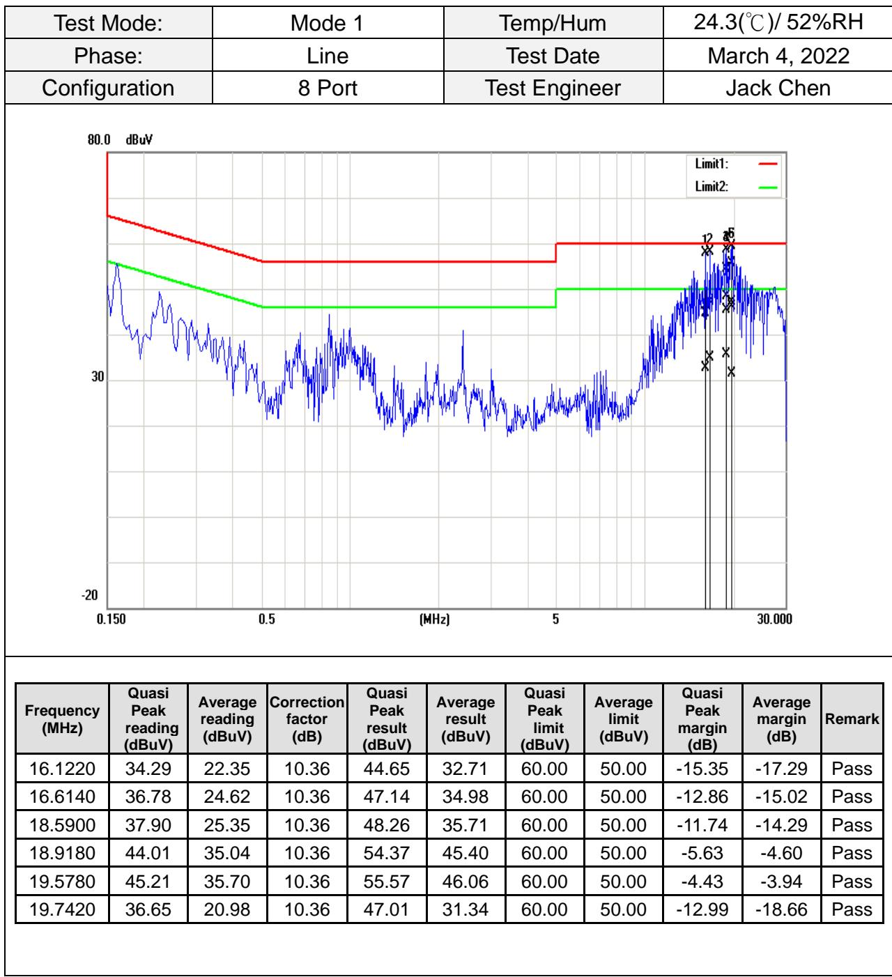
Note: Correction factor = LISN loss + Cable loss.
