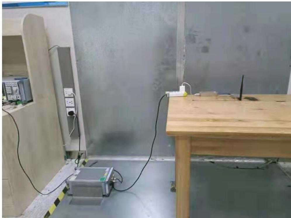
Test Frequency From 30MHz-1000MHz
