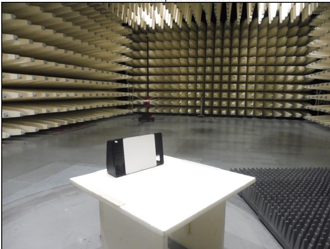
Photo 2: Test setup for radiated emission testing.
