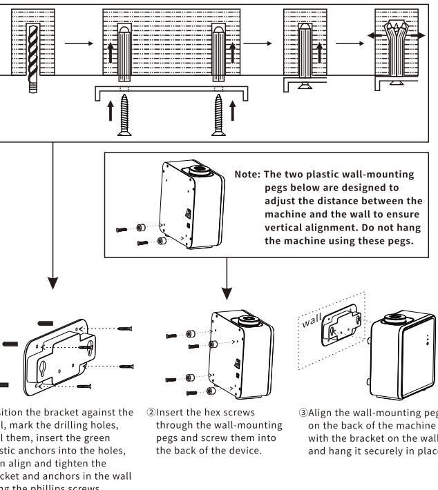
Note: The two plastic wall-mounting pegs below are designed to adjust the distance between the machine and the wall to ensure vertical alignment. Do not hang the machine using these pegs.
