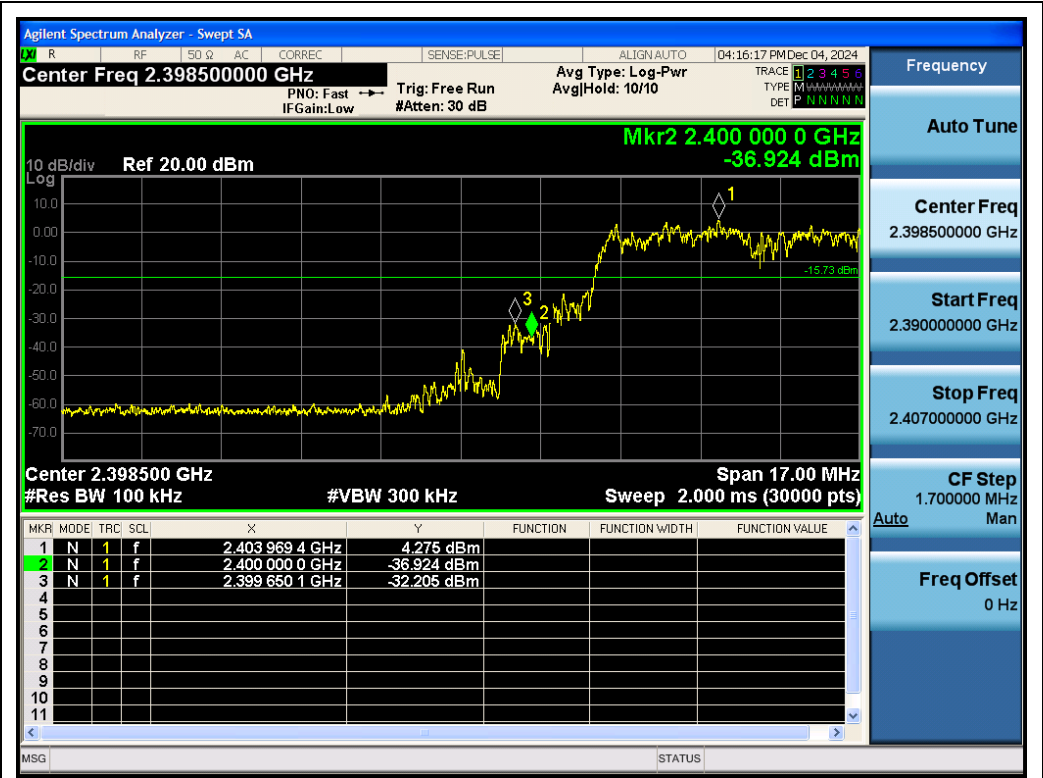
Test_Graph_EDR_HOP_ANT1_NA_2Mbps_Lower Band Edge Emissions
