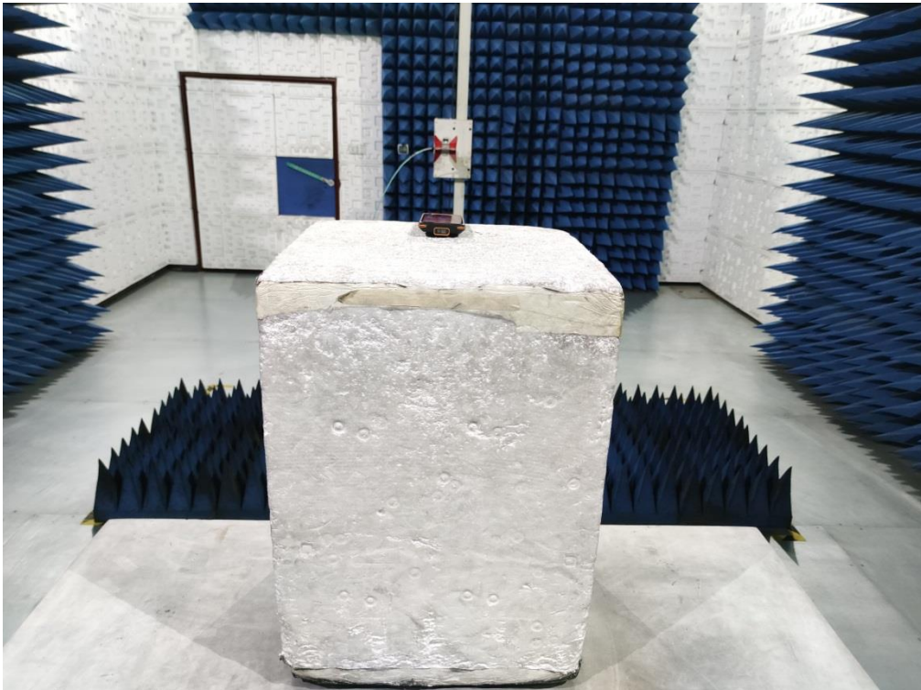
RADIATED EMISSION TEST SETUP ABOVE 1GHz
