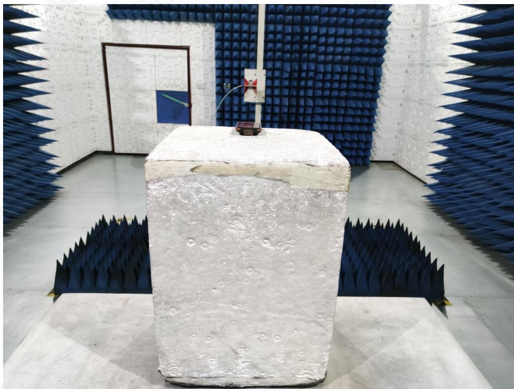
FCC RADIATED EMISSION TEST SETUP ABOVE 1GHZ
