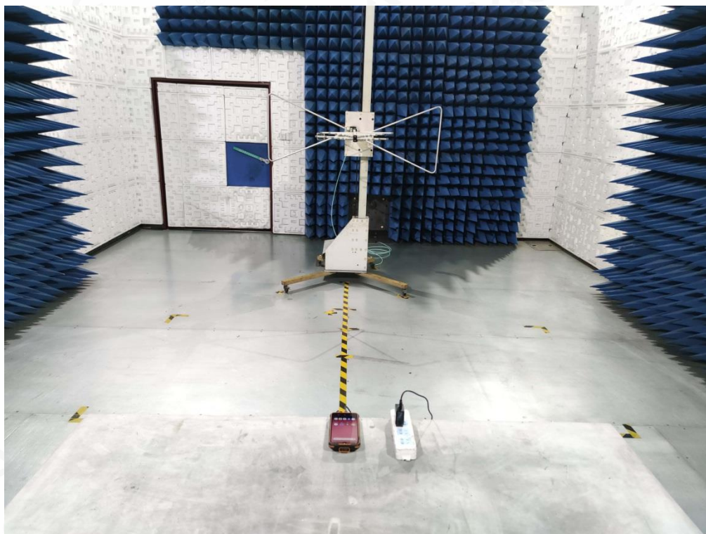
FCC RADIATED EMISSION TEST SETUP ABOVE 1GHZ
