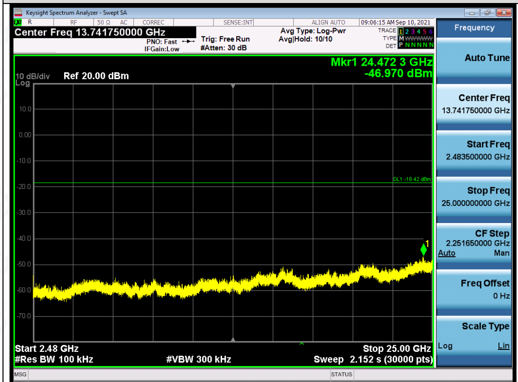
Test_Graph_802.11n20_ANT1_2437_MCS0_Higher Band Emissions
