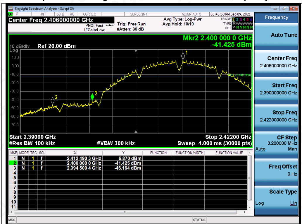
Test_Graph_802.11b_ANT1_2412_1Mbps_Lower Band Edge Emissions
