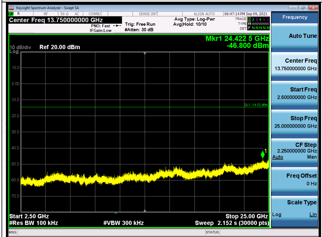
Test_Graph_802.11b_ANT1_2462_1Mbps_Higher Band Emissions
