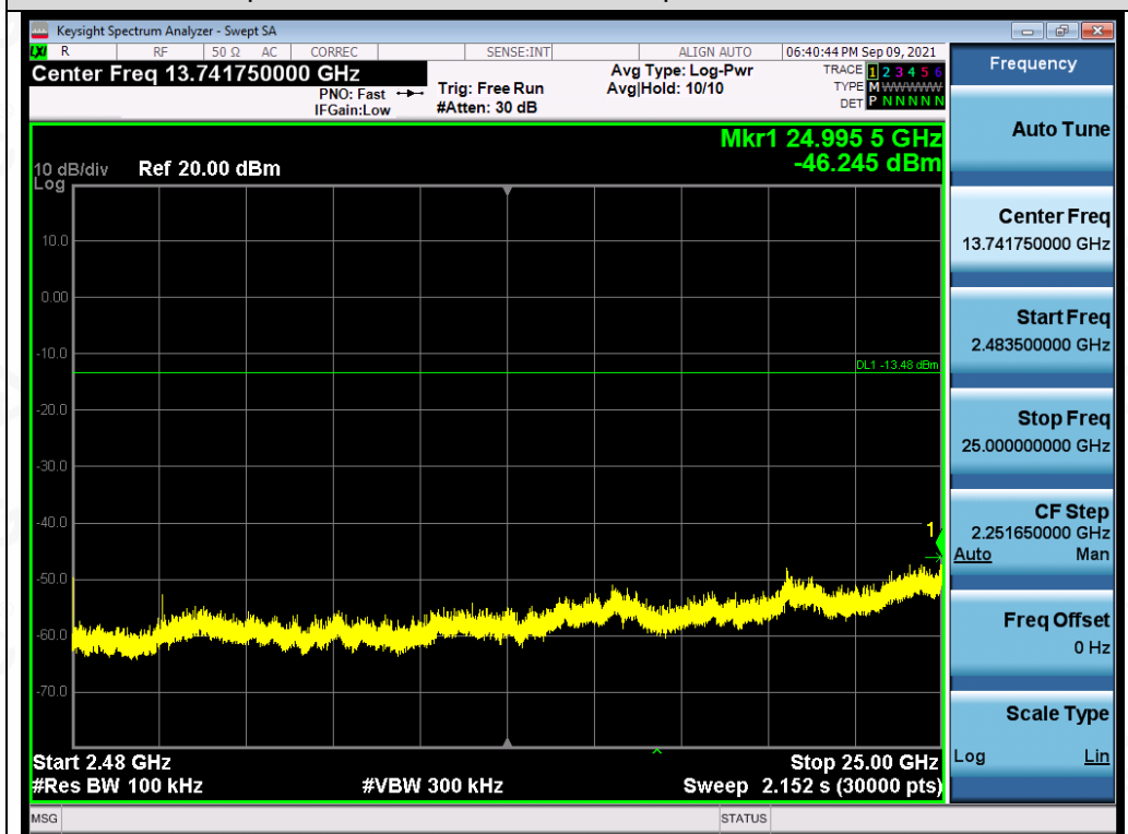
Test_Graph_802.11b_ANT1_2412_1Mbps_Higher Band Emissions
