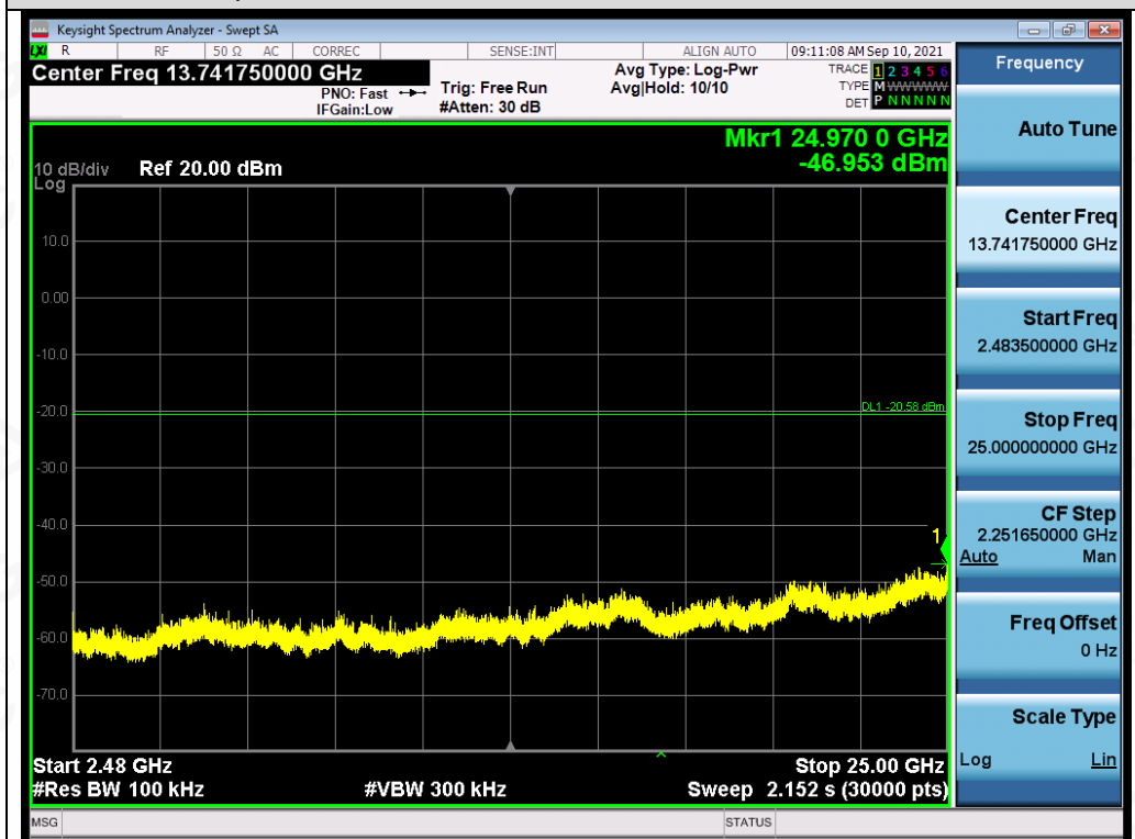
Test_Graph_802.11n40_ANT1_2422_MCS0_Higher Band Emissions
