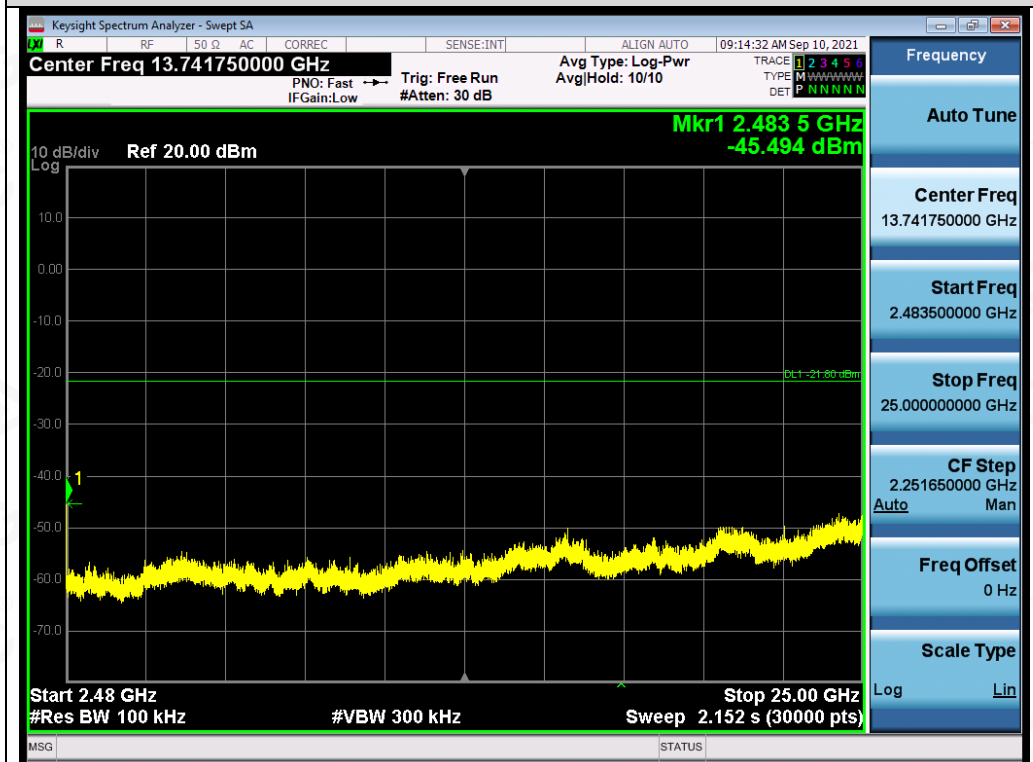
Test_Graph_802.11n40_ANT1_2437_MCS0_Higher Band Emissions
