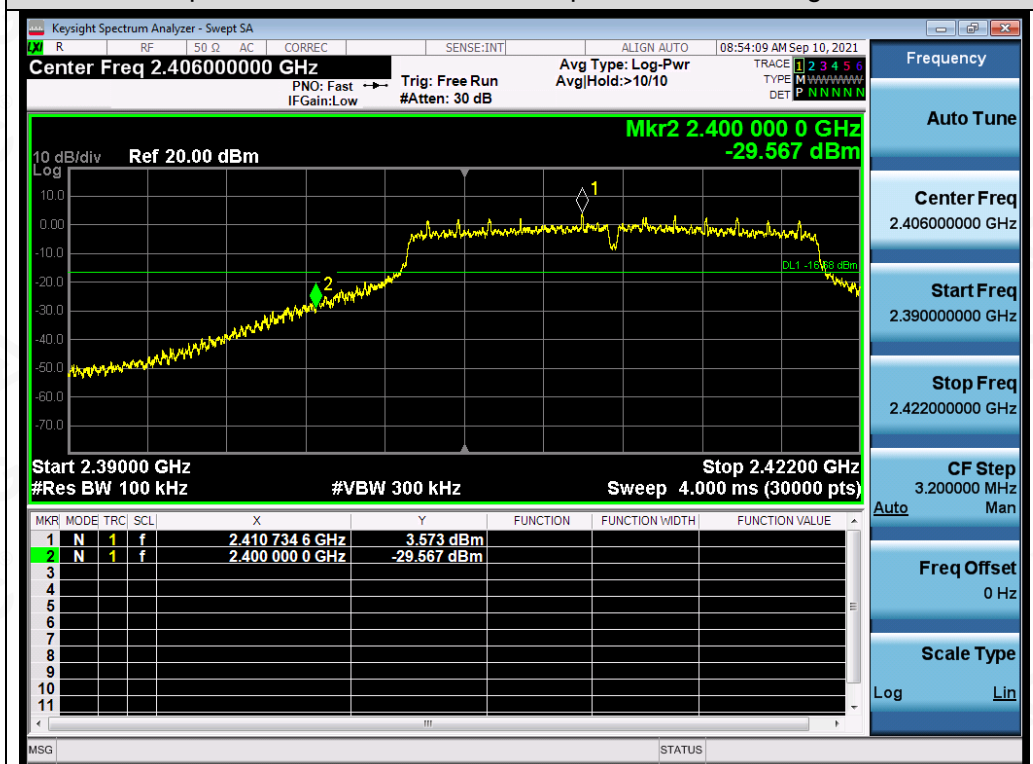
Test_Graph_802.11g_ANT1_2412_6Mbps_Lower Band Edge Emissions
