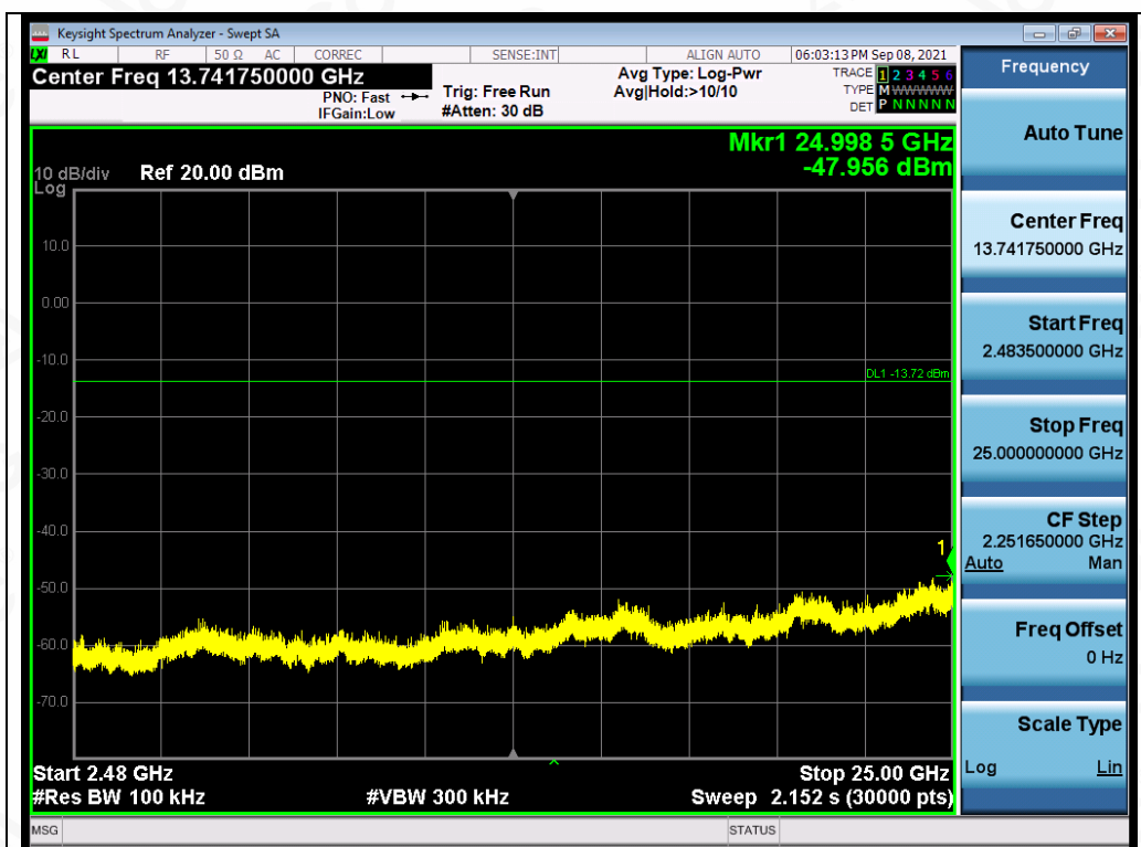
Test_Graph_EDR_ANT1_2402_3Mbps_Higher Band Emissions
