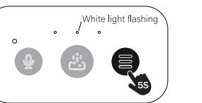
1. Long press the button 5 seconds and white light will flashes to enter the network configuration mode.
